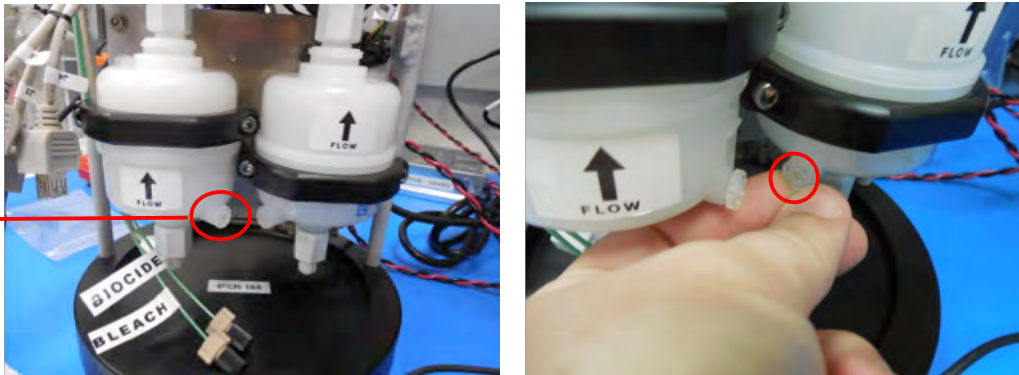
Figure 6.1-2: Left Cartridge – Loosening Fill Port Plug
