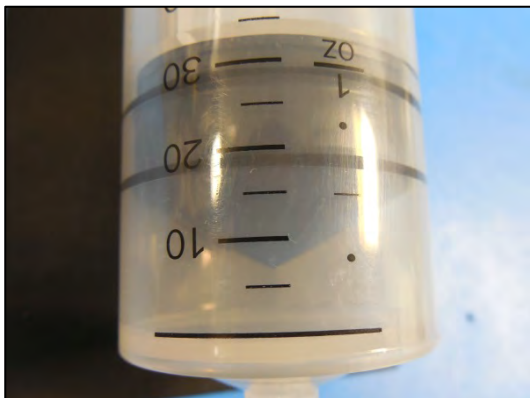
Figure 6.3.3-2: Bead Reservoir with Plunger at 20mL Marker
